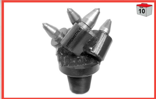
EM312 4 Tooth Pilot, 3-1/2" Pin. Takes #EMC31-HD teeth.
