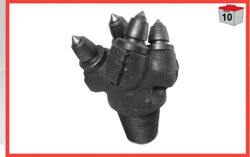
EM238 4 Tooth Pilot, 2-3/8" Pin. Takes #EMSC1-01 teeth.
