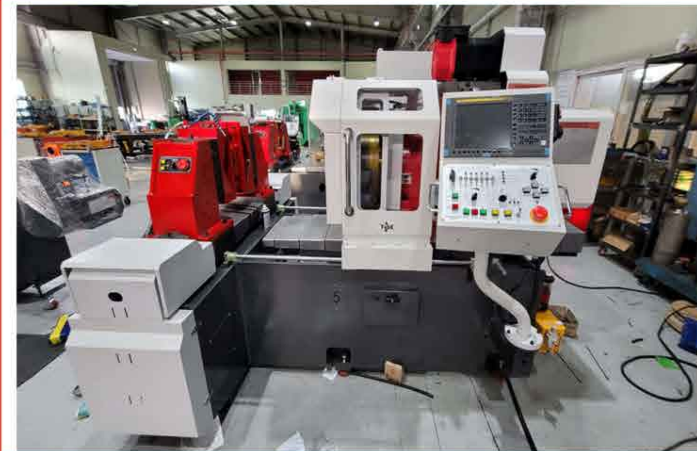
CNC LATHE Up To 20" Threading Capacity
