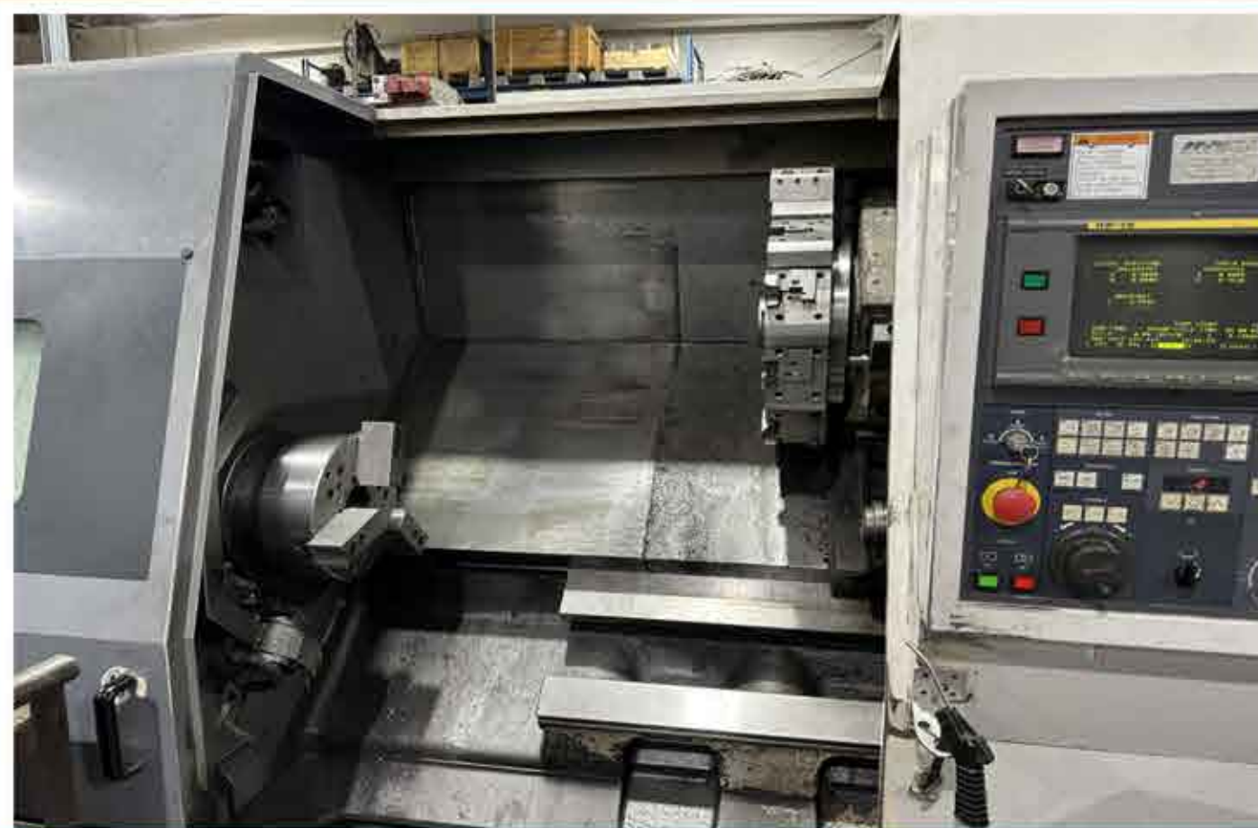
CNC LATHE Max. Turning Diameter: 16.0"
